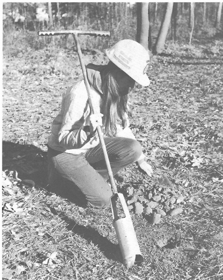
Figure 4. Subsurface testing with a soil auger.
