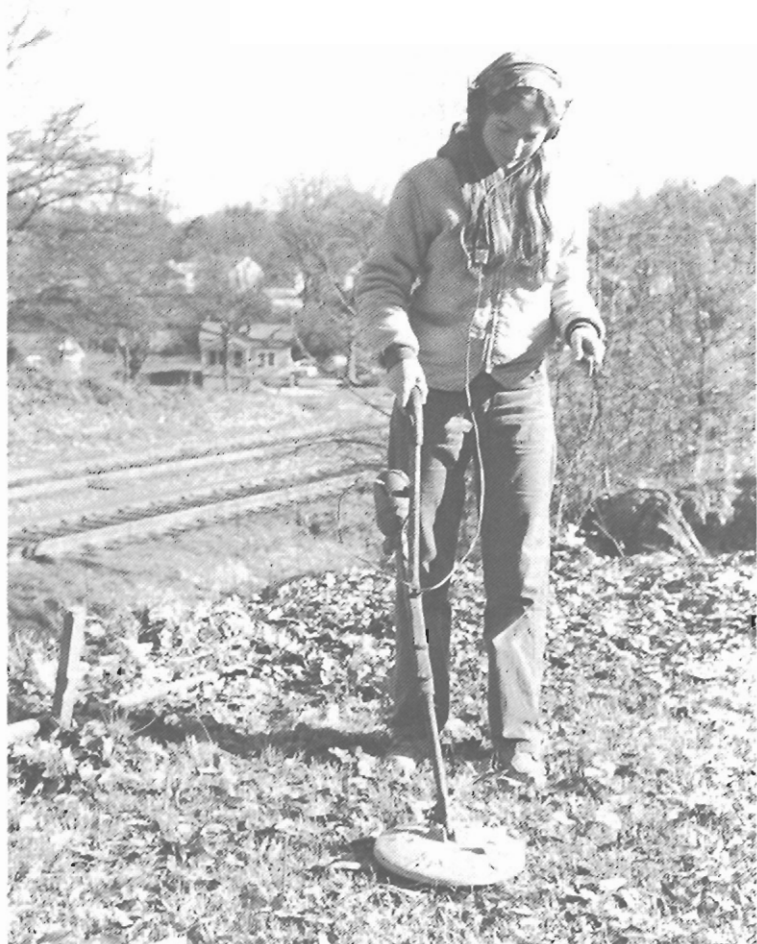
Figure 5. Conducting metal detection survey with the Metrotec Model 220.
